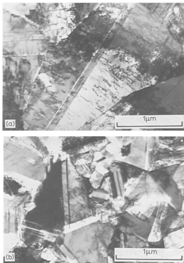
Fig. 2. TEM investigations of a deposit at the \langle 211 \rangle \rightarrow \langle 110 \rangle boundary (duty cycle 60%; pulse frequency 60 Hz). Scale bars: 1 \mu\text{m} . (a) typical \langle 211 \rangle crystallite near the cathode edge; (b) finer grain sized \langle 110 \rangle crystallites at the centre of the disc cathode.
